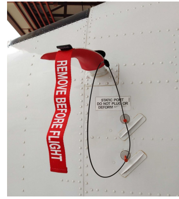
De Havilland DH-6 Twin Otter Pitot Cover, Static Air Plugs
