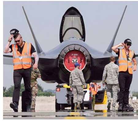
Lockheed Martin F-35 Exhaust Plug, non-folding type
