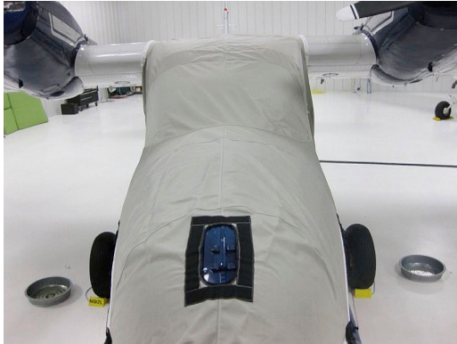
Grumman Widgeon Cockpit/Nose Cover, tie-down cleat detail
