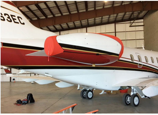
Canadair Challenger 300 Intake/Exhaust Covers, 3-Strap Intake/Exhaust Covers, 3-Strap Type. Successfully installed by two crew, one ladder.
