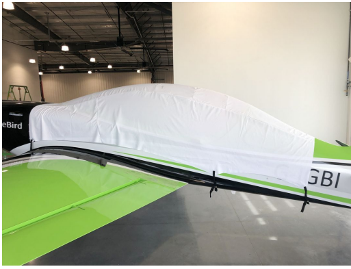
Game Composites GB-1 Canopy Cover, test fit cover
