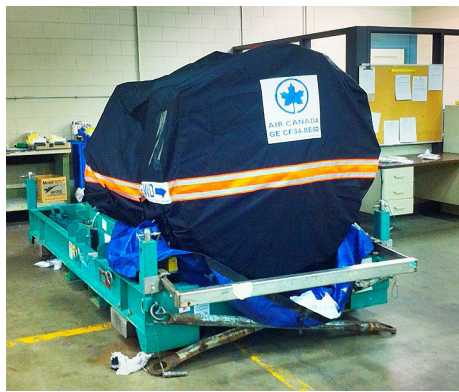
GE CF-34 QEC Engine Long-term Storage/Transport Cover "Bag"
