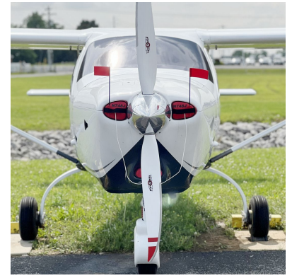
ENGINE PLUGS PREVENT BIRD NEST FOD. Piper Saratoga Engine Cowling Bird's Nest Jabiru J230-SP Engine Inlet Plugs
