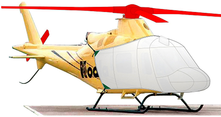
Koala Bubble, Rotor Hub, Blade & Tail Rotor Covers (illustration) Agusta Leonardo A169 Bubble Cover with Wire Strike, 3D model
