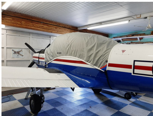
Navion L-17 Travel Cover, Light Weight Canopy Cover (w/out avionics bay extension)
