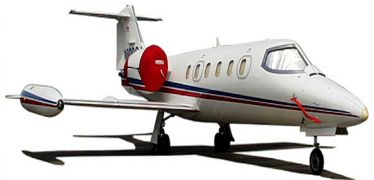
Lear 35 Engine Covers, Pitot Covers & Cockpit HeatShields
