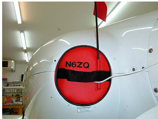
Lancair 320 Engine Inlet Plugs
