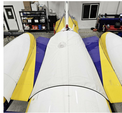
Lear 45 Empennage Saddle Cover W/ Dorsal Inlet Plug (Covers Upper Fuselage Between Pylons, Acm/Apu Area)
