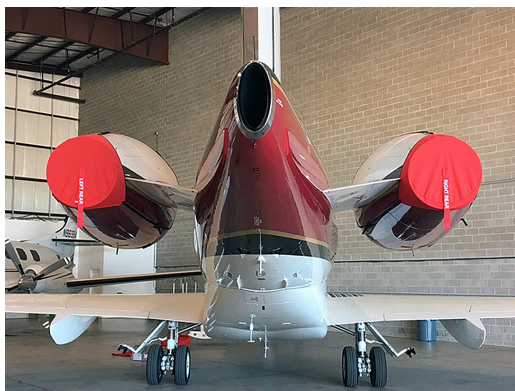
Canadair Challenger 300 Intake/Exhaust Covers, 3-Strap Type
