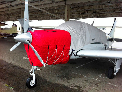
Beech Bonanza Insulated Engine Cover, fully enclosed
