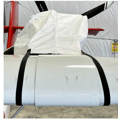
Lockwood Air Cam Engine Cover, test fit cover
