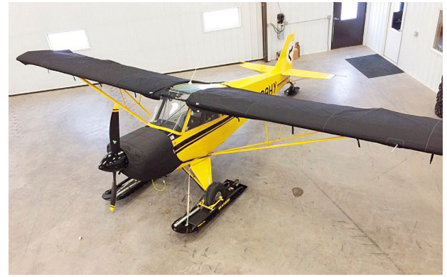
Legend Cub AL3 Insulated Engine Cover with special preheater access vent and attachment detail and fully enclosed under cowling. Aviat Husky Insulated Engine Cover, Wing Covers
