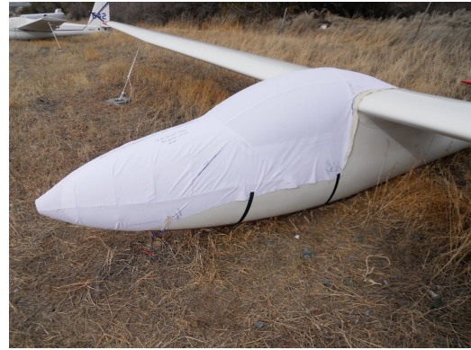
Laister LP-49 Canopy/Nose Cover, test fit cover
