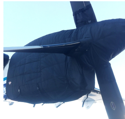
ATR-72-202 Insulated Engine & Prop Hub Covers
