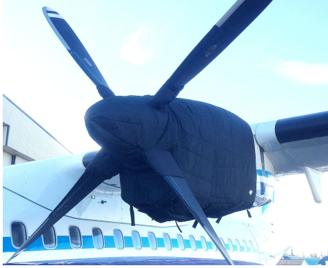
ATR-72-202 Insulated Engine & Prop Hub Covers
