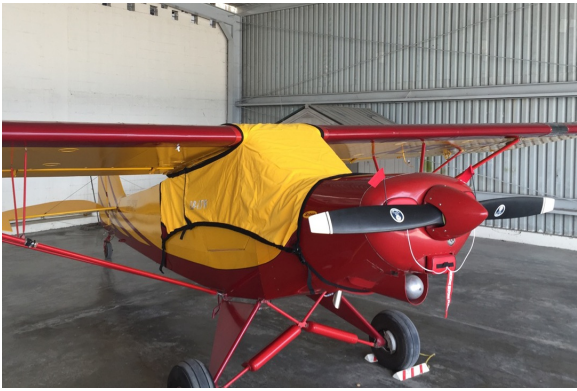
Piper Super Cub Canopy Cover, Engine Plugs ENGINE PLUGS PREVENT BIRD NEST FOD. Piper Saratoga Engine Cowling Bird's Nest
