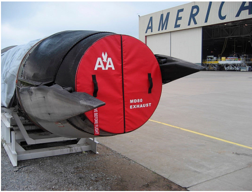
MD80 JT8D Exhaust Plug, Folding Type
