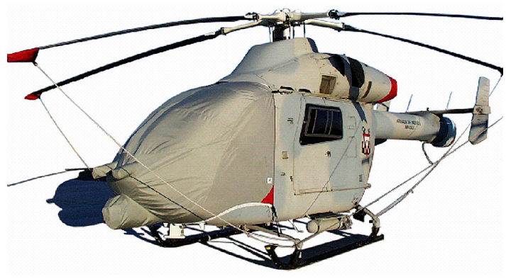
MD900 Forward Bubble Cover (w/Radome), Blade Tie-Downs
