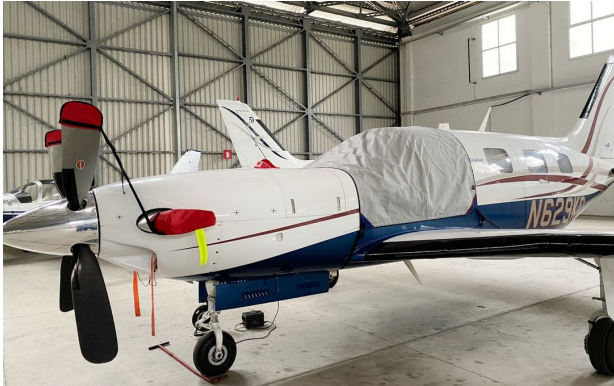
Piper PA-46-500TP Engine Cowling Top Plug
