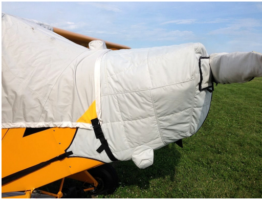
Piper J-3 Cub Insulated Engine Cover with added Pre-heater Piper PA-12 Over-Top Canopy Cover, Engine, Wing & Landing Gear Access Flaps
