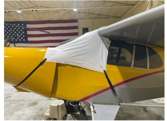
Piper J5A Windshield/Skylight Cover, test fit
