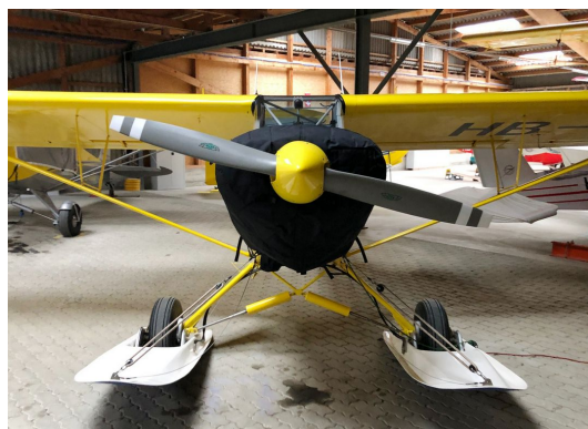
Piper PA-18 Supercub Insulated Engine Cover
