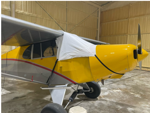
Piper J5A Windshield/Skylight Cover, test fit
