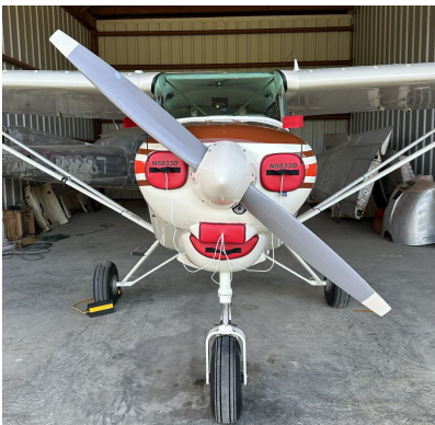
Piper PA-22-150 Engine Inlet Plugs ENGINE PLUGS PREVENT BIRD NEST FOD. Piper Saratoga Engine Cowling Bird's Nest
