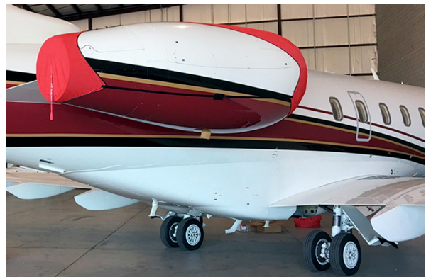
Intake/Exhaust Covers, 3-Strap Type. Successfully installed by two crew, one ladder.
