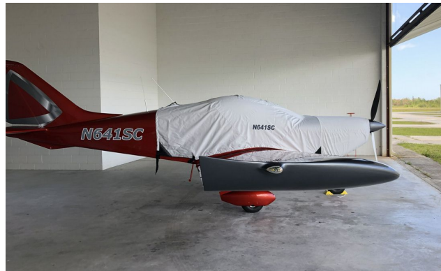
Czech Aircraft Sport Cruiser Extended Canopy/Engine Cover
