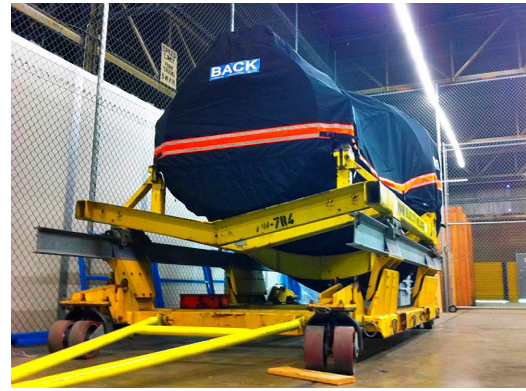
PW 2000 SERIES OFF-LINK ENGINE COVER, "rain cap" style PW JT9D Series Off-Link Engine Transport Cover, Fully Enclosed, P/N: PW-120
