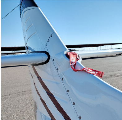
Rockwell Aero Commander 114 Dorsal Inlet Plug
