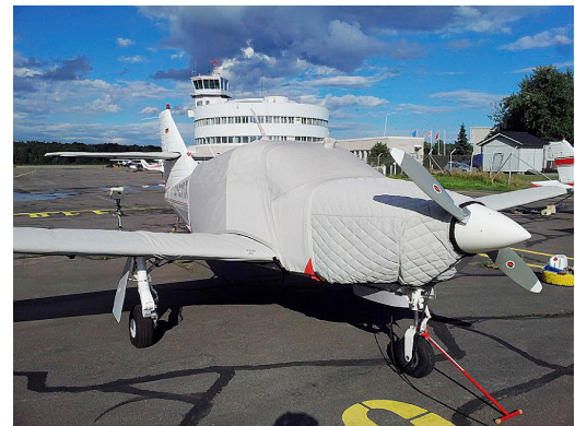
Rockwell Commander 114 Extended Canopy, Insulated Engine, Wing Covers
