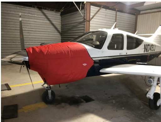
Aero Commander 112 Insulated engine cover
