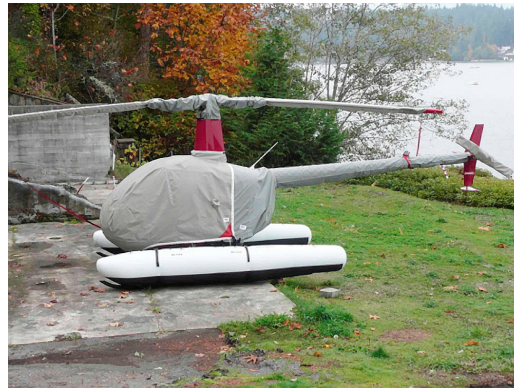
Robinson R-22 Bubble Cover (Ext. Past Rotor Hub), Engine Cover, Tailboom Cover, Blade Covers, Rotor Hub Cover, & Tail Rotor Gear Box Cover
