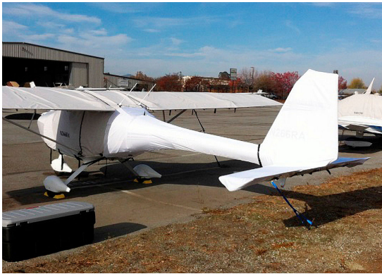
Remos Empennage Cover (test fit cover)
