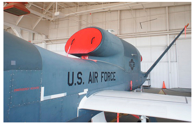
RQ-4/MQ-4 Global Hawk Intake Plug w/ lip (Fits both A & B models & all blocks)
