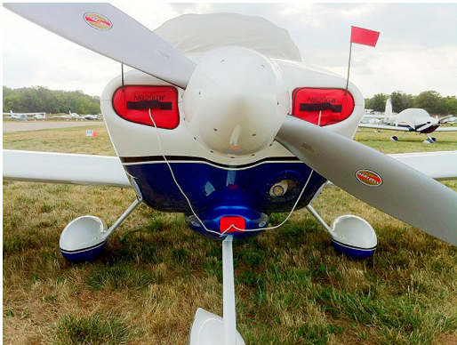
Van's RV-10 Canopy Cover & Engine Inlet Plugs
