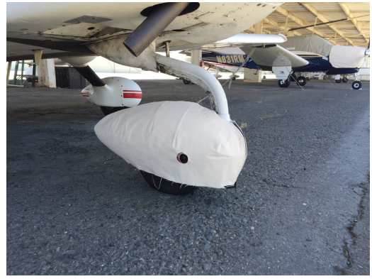
Grumman AA5 Nose Wheelpant Cover, test fit
