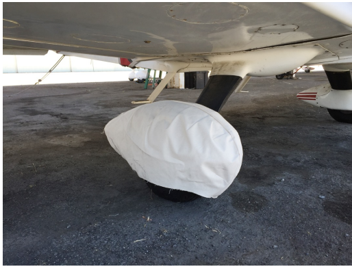
Grumman AA5 Main Wheelpant Cover, test fit
