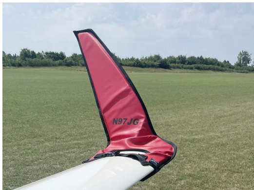
Schempp-Hirth Ventus-2B winglet/wingtip pads
