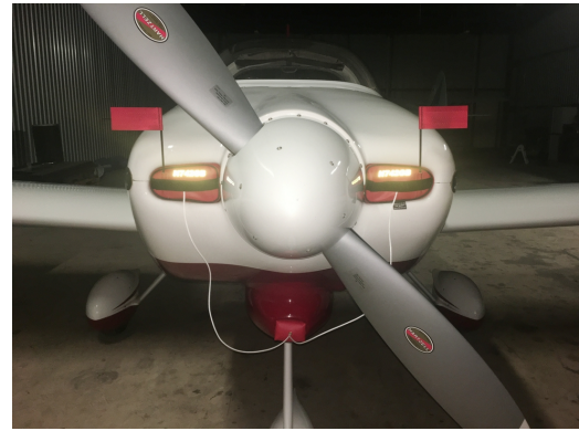
Van's Aircraft RV-7A Engine Inlet Plugs
