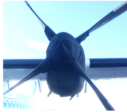
ATR-72-202 Insulated Engine & Prop Hub Covers
