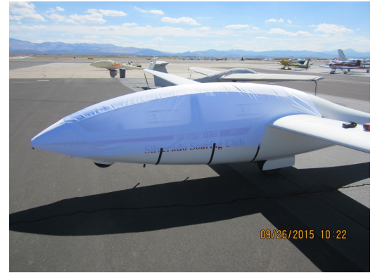
DG-505 Canopy/Nose Cover (test fit cover)
