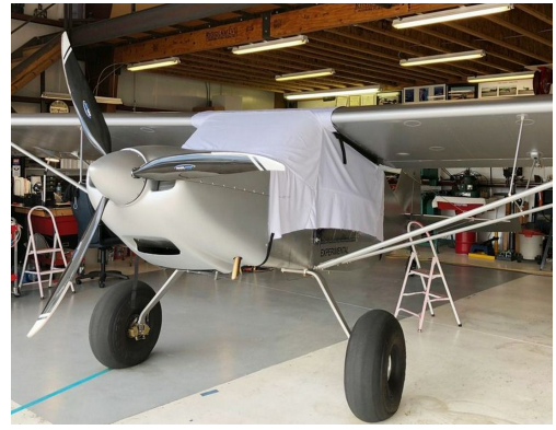
Rans S-20 Canopy Cover, test fit cover
