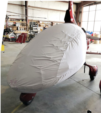
Cavalon Gyrocopter Bubble Cover, test fit cover
