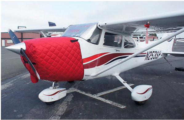
Cessna 172 Insulated Engine Cover, fully enclosed
