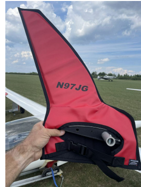
Schempp-Hirth Ventus-2B winglet/wingtip pads
