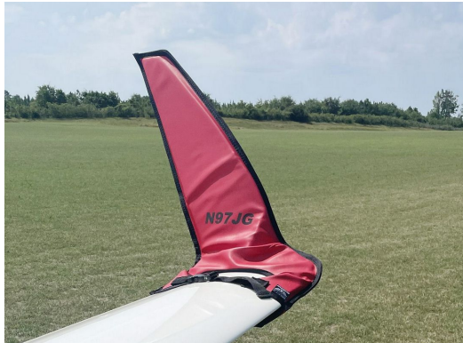
Schempp-Hirth Ventus-2B winglet/wingtip pads
