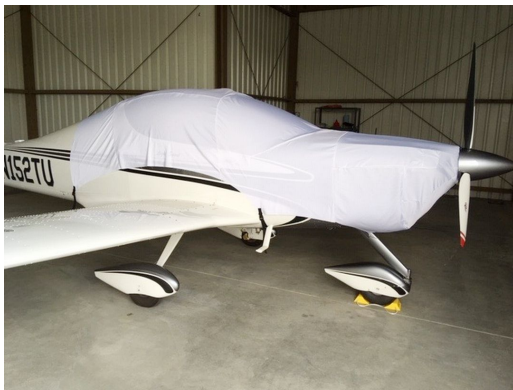
Tecnam Astore Canopy/Engine Cover, test fit cover
