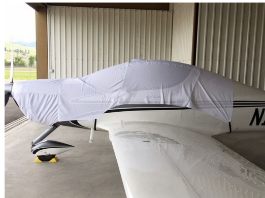
Tecnam Astore Canopy/Engine Cover, test fit cover
