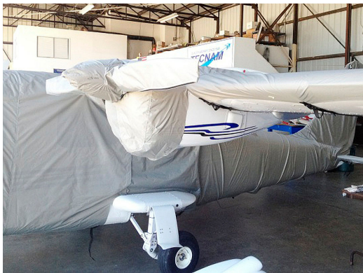
Tecnam Twin Canopy/Nose, Empennage, Wing/Engine, & Propellor/Spinner Covers
