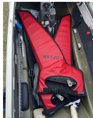
Schempp-Hirth Ventus-2B winglet/wingtip pads
