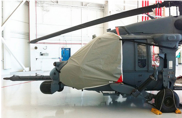
Sikorsky UH-60 Intake/Exhaust Cover Set (IR suppressors)
