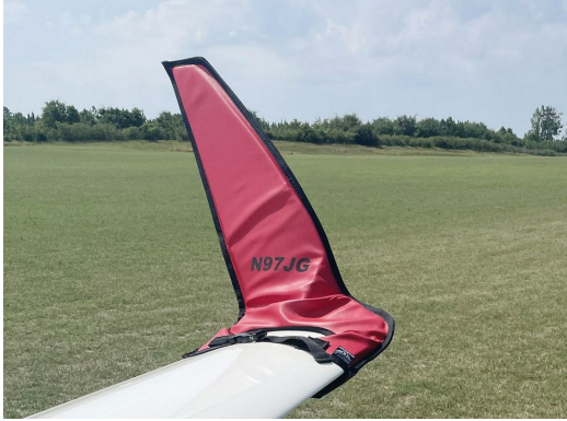
Schempp-Hirth Ventus-2B winglet/wingtip pads
