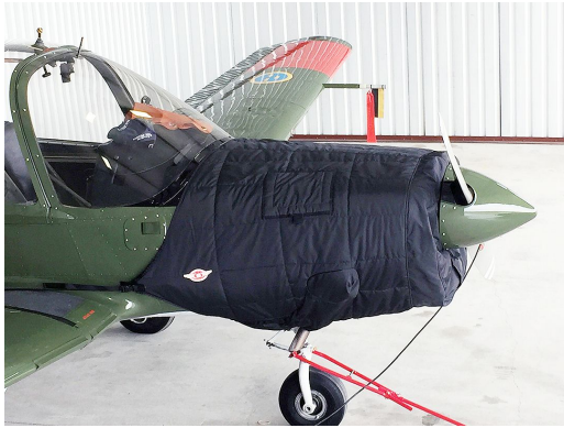
Scottish Aviation Bulldog Insulated Engine Cover
