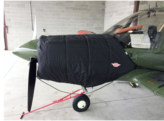
Scottish Aviation Bulldog Insulated Engine Cover
